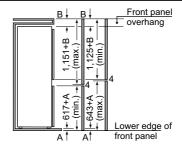
The specified unit door dimensions are valid for a door gap of 4 mm. If a different gap width is used (max. 14 mm), the dimensions
