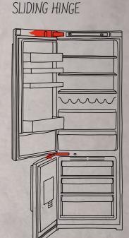
Additional space is required on the inner side of the cabinet to make way for the door hinge.
