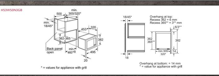
Measurements in mm. The line drawings featured in this brochure are adjusted to the management of the
