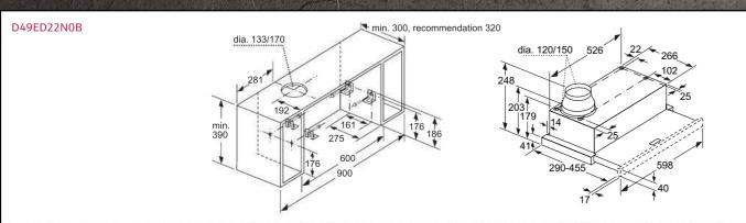
Measurements in mm. The line drawings featured in this brochure are provided as a guide to general dimensions only and are subject to amendment without prior not
