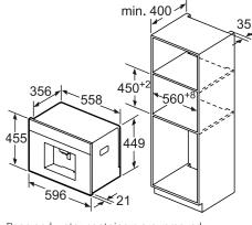
Bean and water containers are removed from the front. Recommended installation height 95-145cm.
