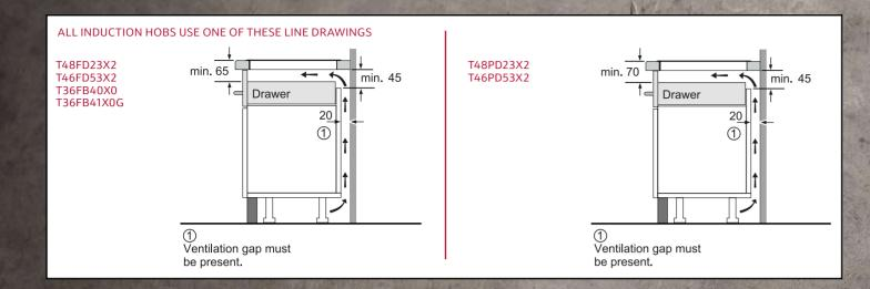
ALL INDUCTION HOBS USE THESE LINE DRAWINGS T48PD23X2, T46PD53X2, T48FD23X2, T46FD53X2, T36FB40X0, T36FB41X0G <del>- -</del> Built-in cooker/ built-in oven ① Ventilation gap must be present
