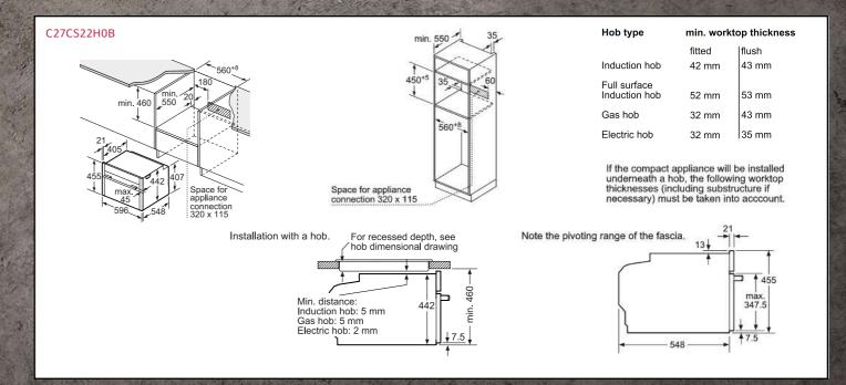
Measurements in mm. The line drawings teatured in this brochure are provided as a guide to general dimensions only and are subject to amendment without prior notice. For full dimensions and in its stallation details loses are refer to the documentation supplied with the appliance.
