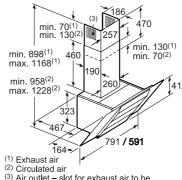
(3) Air outlet – slot for exhaust air to be mounted facing down
